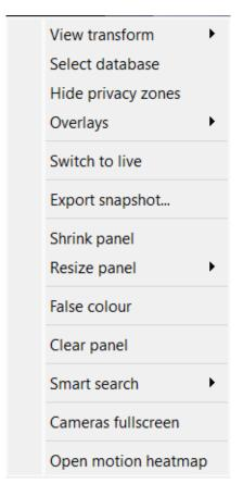
**View transform:** Allows transforming images for cameras with special lenses. (For example, 360-degree cameras.)
